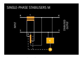
T = series transformer (booster R = variable autotransformer C = electronic control circuit M = servomotor
