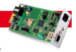
The NetMan 204 Solar board allows the management of a inverter directly linked to a 10/100 Mb LAN with standard network protocols (TCP /IP, HTTP HTTPS, SSH, SNMPv1 and SNMPv3).
